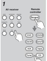
Use the AV receiver's input selector buttons to select an input source.
